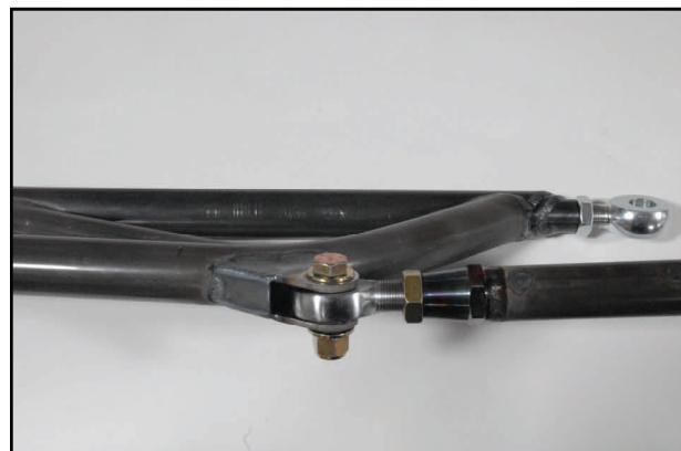
Attach the lower solid rod end to the bottom of the housing using one of the  $2\frac{1}{4}'' \times 3/4''$  bolts, washers and nylock nuts. It's not necessary to tighten hardware completely at this time, the housing will need to be removed later for final assembly.
