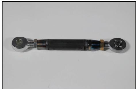
Thread the jam nut on the right hand heim all the way. Lubricate the threads and thread the heim into the slider tube fully. Tighten the jam nut against the slider tube.
