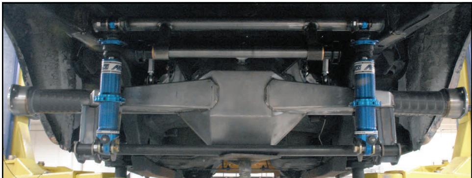
This kit is designed for Fox body owners wanting to run a bigger rear tire, upgrade from the stock rear suspension, also allowing the possibility of mini tubing the rear wheel openings. It allows for greatly increased suspension adjustment at the housing. The included anti roll bar allows the racer to preload the rear suspension for differing track conditions. Also included are adjustable coil over shock mounts, adjustable shocks & their springs are available at an additional cost.
