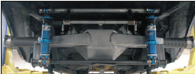
**NOTE:** the housing will need to be squared in the vehicle, ride height and pinion angle will need to be set before the driveshaft is measured. Weight must be on all 4 wheels as well.
