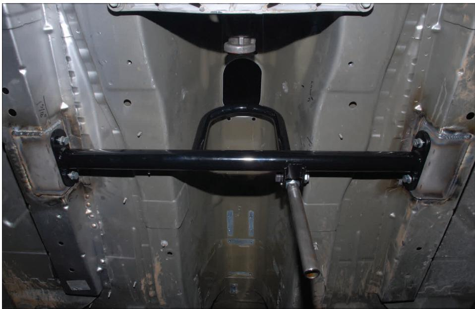
Double check the cross member assembly is at  $25 \frac{1}{4}$ " to the back of the adapters on both sides and tack weld. This assembly welded in completely once all clearance issues on the front of the torque arm are met.
