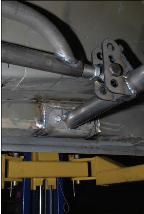
The lower shock mounts attach approximately mid point on the adjustable housing mounts. There are 2 left hand brackets and 2 right hand brackets. One each attach to each of the adjustable housing mounts.
