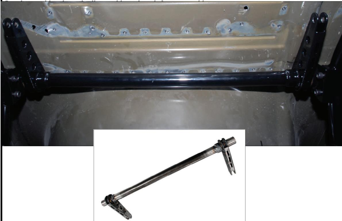
Push the 2 oillite bushings into the bushing mounts making sure they slide freely into the mounts. Lightly grease the inside of the bushings with bearing grease. Slide the bushing assemblies onto the anti roll with the thrust surface of the bushing facing in. The bushing assembly must slide onto the anti roll freely, it may be necessary to sand any powder coat or paint off the ends of the anti roll to allow the bushing assemblies to rotate freely on the ends of the anti roll bar.
