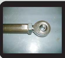
Install the heim joint into the slider tube. There should be only 2 to 3 threads showing between the rod end and the jam nut. Use an anti seize lubricant or a heavy grease to prevent on the threads to prevent them from galling during assembly. It is imperative that you tighten the jam nut securely against the slider tube to prevent the heim from backing out of the tube.
