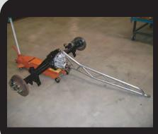
Bolt the torque arm to the housing using the <sup>3</sup>/<sub>4</sub>" bolts, nuts and washers supplied in the kit. Make sure you use the supplied washers so the bolts will tighten properly against the housing brackets. You may need to grind the corner of the lower nut slightly to clear the housing. At this point the housing and torque arm assembly can be set on the floor jack, it's ready for installation.
