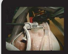
On 3 channel brake applications the electrical connection for the sensor is located on top of the rear end housing. Release the safety catch on the weather pack connector and remove from sensor. Slide the strain relief from the bracket.
