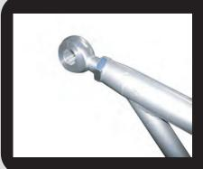
Install the solid rod ends into the torque arm adjuster and the top tube adapter in the torque arm. Set the jam nuts on the rod ends at 7/8" as you did on the adjuster. Thread the rod ends into the tube until the jam nut touches the tube adapter and adjuster. Again, use anti seize on the threads. Do not tighten the jam nuts at this time. This will be done after the pinion angle is set.
