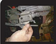
Remove the emergency brake cable from the actuator. This procedure may vary slightly depending on the year of your car. On drum brake equipped models you will have to remove the entire cable assembly from the vehicle leaving it attached to the rear end. Aftermarket cables may be needed during assembly depending on which brake kit is used.
