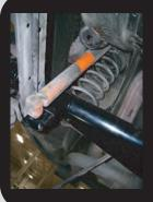
Carefully jack the housing up into the car first inserting the coil springs into their respective pockets. Make sure the tops of the springs are properly indexed into the rubber insulators. Once the rear end housing is jacked up into the car, install the lower control arm bolts & nuts, lower shock mount studs & nuts.
