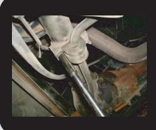
Remove the nuts from the u-bolts that attach the sway bar bushings to the axle tubes. If you are re-using the original sway bar you must purchase 2, 3" muffler clamps and elongate the holes in the bushing strap to accommodate the bigger clamp.
