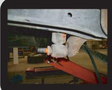
Turn the lower shock studs forward so that they do not catch on the rear end as it is lowered from the vehicle.
