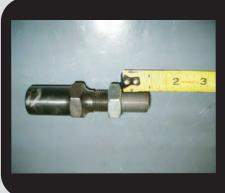
Start with the installation of the lower adjuster in the bottom of the torque arm by threading the jam nut on the adjuster (7/8"). As mentioned earlier use an antiseize lubricant (not supplied) on the thread to prevent galling during assembly. Insert the adjuster into the lower tube adapter of the torque arm until the nut touches the tube adapter, do not tighten the jam nuts at this time.
