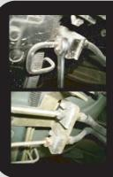
Disconnect the brake line where the hard line attaches to the rear brake hose on the body. On models with 4 channel ABS there will be 2 lines, 1 to each corner of the vehicle.
