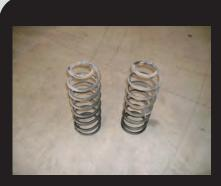
At this point you will need to lower the rear end assembly just enough to get the coil springs out of the vehicle. Be extremely careful during this part of the disassembly, the coil springs are under an extreme amount of tension! Once the rear end has been dropped from the car enough to remove the springs slide them from their pockets.
