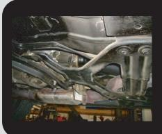
Remove the tunnel brace. On convertible models the brace is attached to the crossmember and the body. With these models it is recommended to use an aftermarket tunnel brace.
