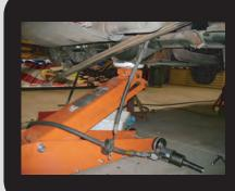
At this point it will be necessary to support the rear end with a floor jack. Raise the rear end just enough to unload the rear shocks being careful not to upset the vehicle on the jack stands..
