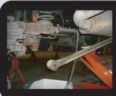
Remove the bolt attaching the panhard bar to the rear end. It may be necessary to pry the panhard bar from the mount.
