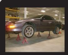
The vehicle must be supported by the chassis structure as close to the corners as possible. Support the vehicle near the forward lower control arm pockets in the rear and the suspension mounting points in the front. Do not support the vehicle by any suspension components. This must be done on a hard, level surface.
