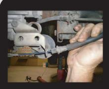
On disc brake models you will have to release the 3 retaining clips that attach the emergency brake cable housing to the caliper bracket. Caliper brackets vary from year to year but the cable housing attaches the same. Removing the cable housing from the bracket allows you to leave the brake assemblies attached to the rear end, they can be removed once the rear end is removed from the vehicle if you are planning on reusing your original brake assemblies.
