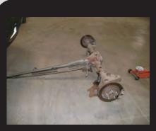
Slide the rear end from underneath the car. As you do this the torque arm will slide out of the clamshell mount on the side of the transmission and drop towards the ground. At this point carefully lower the rear end as near to the ground as possible allowing you to roll the assembly out from underneath the vehicle.
