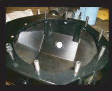
It's time to prep the housing for installation! It's important to clean the housing thoroughly of any debris that might be left behind. You can clean the tubes by shoving a rag through them with a broom handle. Any debris left behind can potentially cause premature gear or bearing failure!
