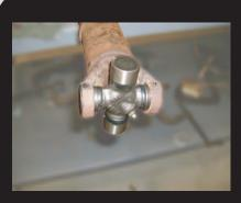
If you plan on reusing your stock driveshaft you will need to use a conversion u-joint. We offer some conversion u-joints, but all can be found at a local parts store. If you do not have the proper tools to change the u-joint a competent machine shop can handle this task for you.
