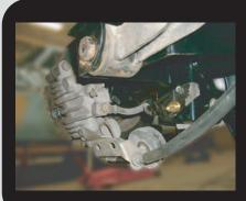
Install the panhard bar, sway bar and their associated hardware. At this point you can also reattach the brake lines, emergency cables (if so equipped) and 4 channel ABS harness (if applicable).
