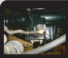
On some applications it may be necessary to drill a small hole in the back of the lower control arm mount for the caliper brake hose attachment. This procedure is easier to do when the rear is out of the vehicle.
