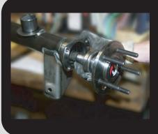
Install the axle seals (where applicable) using a suitable driver. Make sure that they are inserted deep enough to clear the bearing retaining ring.
