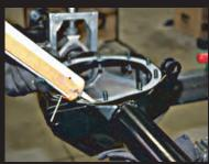
Use a small bead of silicone where the center section touches the gasket. Install the center section. You may need to use a block of wood and a hammer to get the center section to slide over the studs the first time. This helps with stud alignment. Use the nuts and washers supplied in the kit. Tighten the nuts in a criss-cross pattern. They will need to be tightened to 40 ft. lbs.
